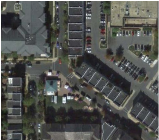
Thoroughfares with speeds of 30 m.p.h. or less, may have offset intersections, or, occur at angles as means of calming traffic as shown in this example in Kentlands, Gaithersburg, Md.
